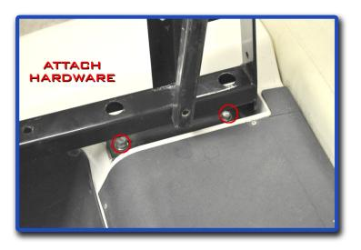
Attach bagwell brackets to the floor of the bagwell using hardware from pack 2. Attach bagwell bracket to main bracket using hardware from pack 2.
